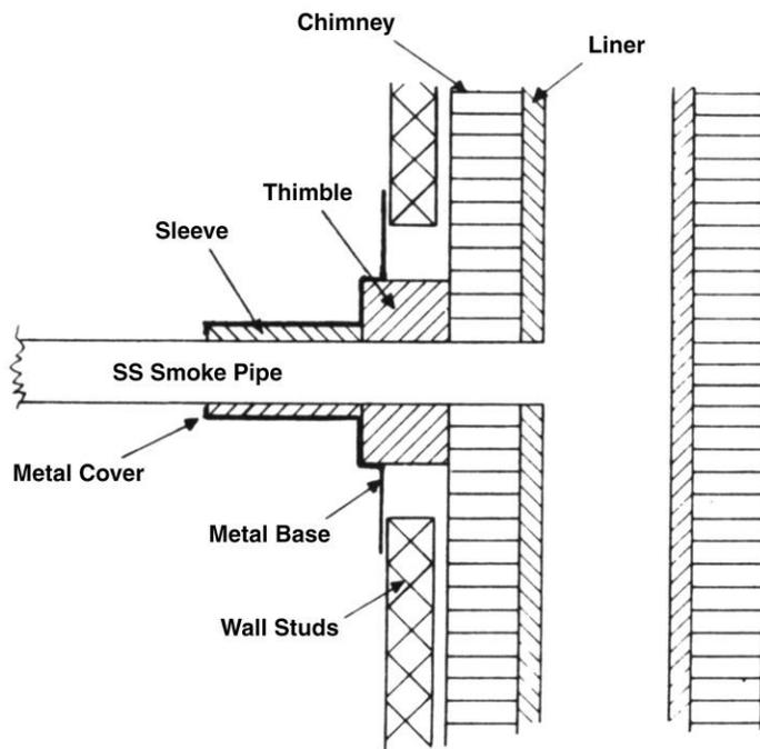
**Figure 8: Wall Cross Section**
