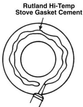
**Figure 7: Applying Cement**
