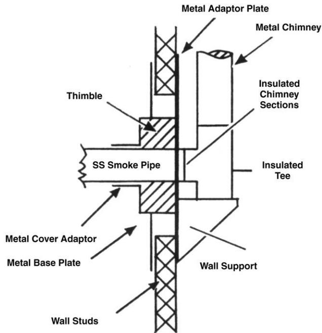
**Figure 11: Wall Cross Section**
