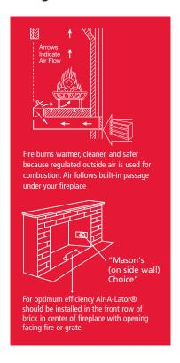
Exclusive Dual Damper System gives you complete control of combustion air. Other outside air intakes just let you control the volume of air. The Air-A-Lator® Dual Damper System gives you control not only of volume of air, but it also lets you control the direction of air. Both are necessary to produce the proper flames and control the rate of burning.
